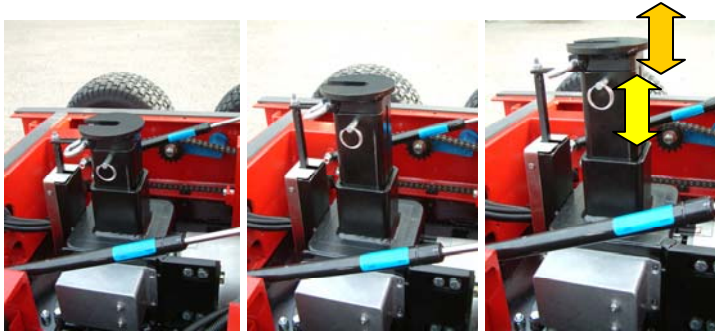
Heavy duty electrical lift with additional mechanical extension.
