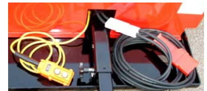
Cable storage section
