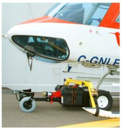
Quick connect Jack head on V201 allows for instant attachment exchange from one to the other (AT44 to AT45)
